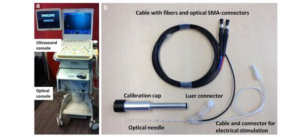
Fig. 3 Picture of the optical console (left) and the optical needle (right) used in the measurements
