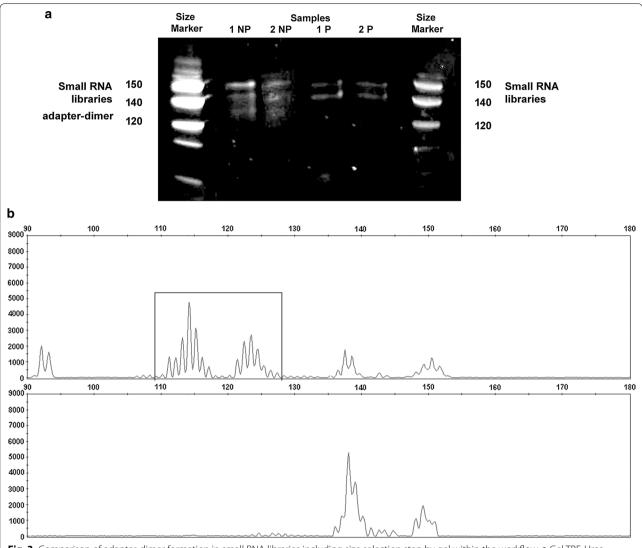
**Fig. 3** Comparison of adapter-dimer formation in small RNA libraries including size selection step by gel within the workflow. **a** Gel TBE-Urea staining showed the presence of adapter-dimer (around 120 nt in size) in non-purified (NP) samples, and it was removed in purified (P) samples 1 and 2. **b** Electropherogram showed elimination of adapter-dimer (black box) from the purified exosomal cDNA library, and an increase in the small RNA library amount
