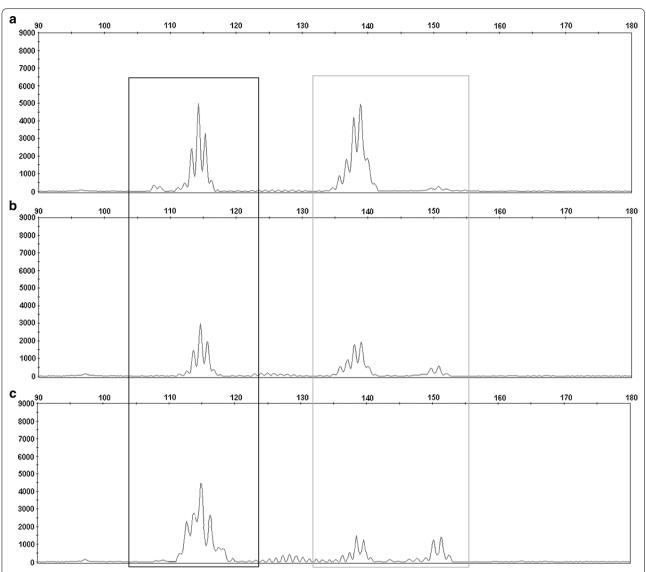
**Fig. 2** Electropherograms obtained for DNA fragment analysis by capillary electrophoresis to analyze adapter-dimer formation. Three different cDNA libraries from urinary exosomal samples showed the presence of adapter-dimer (black box), high amount of adapter-dimer with high cDNA library (grey box) (**a**), low amount of adapter-dimer with low cDNA library (**b**), and high amount of adapter-dimer with low cDNA library (**c**)
